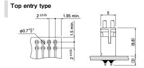
Note: 1. The above figure is the figure viewed from soldering side.
