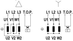
Note: Change of rotation direction by reversing two phases
