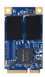
SV240-300 utilizes 3D NAND for higher capacity up to 1920GB and provides more power efficiency than 2D NAND. Regarding reliability, SV240-300 is implemented with LDPC (Low Density Parity Check) ECC engine to extend SSD endurance and increase data reliability while reading raw data inside a flash chip. In addition, the drive comes with various implementations including powerful hardware ECC engine, power saving modes, wear leveling, flash block management, S.M.A.R.T., TRIM, and DataDefender™.
