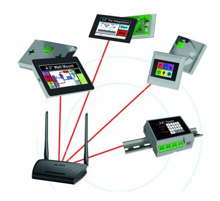
So distance from Core to Satellite Display may not exceed 10m. Alternatively WiFi signal is amplified by repeater.
