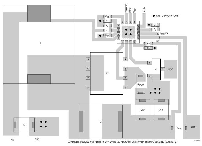
Figure 5. Boost Converter Suggested Layout
