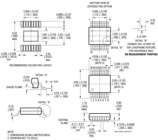
MSE Package 16-Lead Plastic MSOP, Exposed Die Pad (Reference LTC DWG # 05-08-1667 Rev A)
