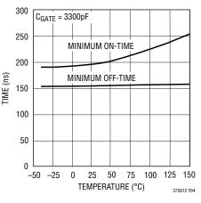
Figure 4. Typical Minimum On and Off Pulse Width vs Temperature
