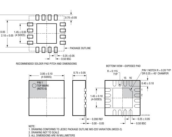
UD Package 16-Lead Plastic QFN (3mm × 3mm) (Reference LTC DWG # 05-08-1691)
