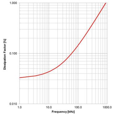
Test Equipment: E4991A or equivalent
