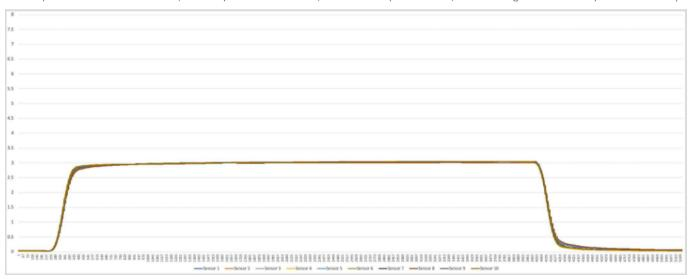
Test results: 2 hours ventilation, range drift <20ppb;
