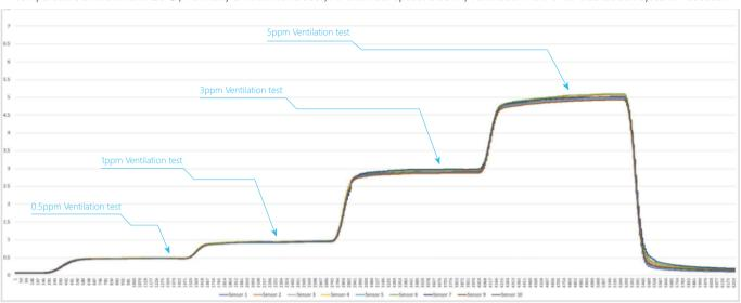
Test result: 0-5ppm linear error <± 3%; 5-10ppm linear error <± 5%;
