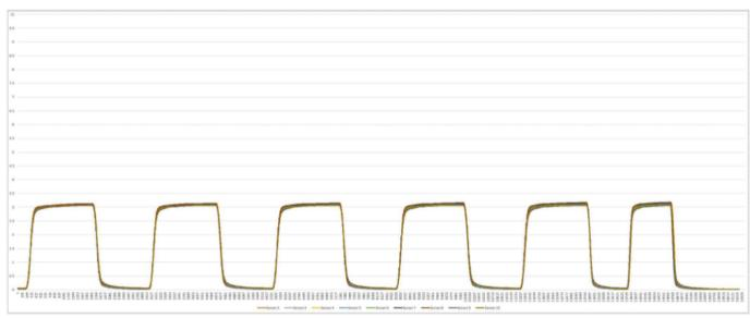
The test results show that the repeatability error range is <20ppb (5ppm ± 1% of full scale is the normal range);
