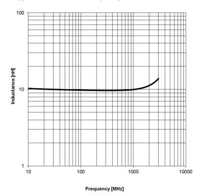
DESCRIPTION Projection **WE-CAIR Air coil** Würth Elektronik eiSos GmbH & Co. KG EMC & Inductive Solutions Max-Eyth-Str. 1 Order.- No. 74638 Waldenburg COMPLIANT SIZE Germany Tel. +49 (0) 79 42 945 - 0 744911098 www.we-online.com A4 2014-10-27 SSt 1.0 HBH eiSos@we-online.com REV BY Size: 1340 DATE CHECKED
