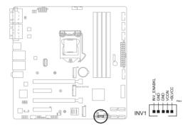
**IMPORTANT!** The backlight inverter power header supports 1A current to the maximum.
