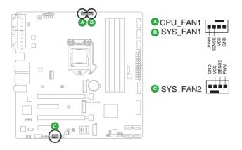
**CAUTION!** Do not forget to connect the fan cables to the fan headers. Insufficient air flow inside the system may damage the motherboard components. These are not jumpers! Do not place jumper caps on the fan headers!
