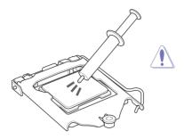
**CAUTION!** Apply the Thermal Interface Material to the CPU heatsink and CPU before you install the heatsink and fan if necessary.
