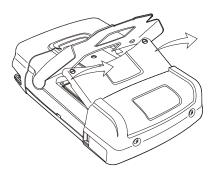
Figure 43. Removing the Battery Cover
