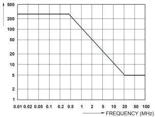
Figure 46. Max. Input Voltage vs. Frequency
