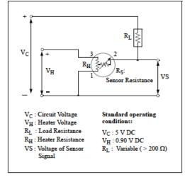
Fig 2. Standard circuit
