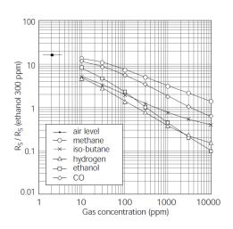
Fig3. Sensitivity characteristics
