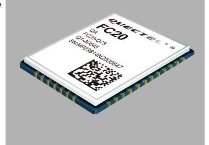
FC20 is a new embedded Wi-Fi and BT wireless communication module featuring high performance and low cost. Designed in ultra-compact 16.6×13.0×2.1mm profile, FC20 module can effectively optimize size and cost for end-products, which totally meets customer requirements on size sensitive applications to the maximum extent.
