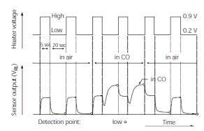
Fig 2 SB-95-12: Operating conditions and output signal
