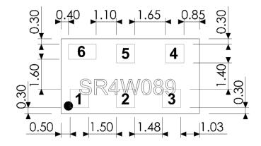
1-5 copper pads: 1.0 x 1.0 (mm) 6 copper pad: 1.5 x 0.8 (mm)
