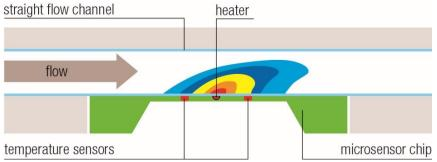
Due to the small size of the sensor chip and the very thin flow channel wall (≤100 um), even the slightest deposition can cause measurement deviations. Depending on the kind of deposits, a few micrometers might be sufficient to cause considerable measurement deviations. These deposits may be permanent (i.e. mineral or salt deposits) or transient (layer of previous liquid among alternating media types).
