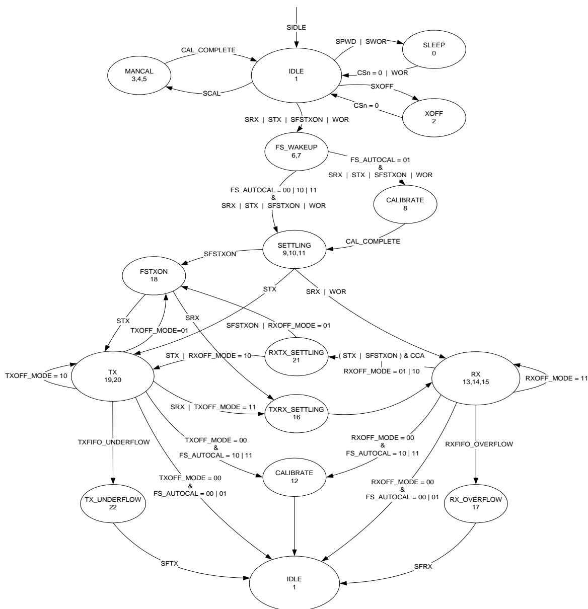
Figure 25: Complete Radio Control State Diagram
