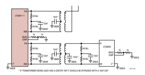
Figure 50. Interfacing an LTC6811-1 with a μC Using an LTC6820 for Isolated SPI Control
