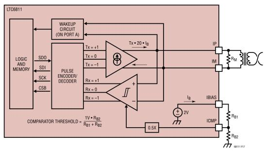
Figure 17. isoSPI Interface
