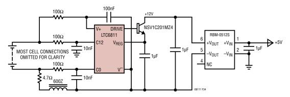
Figure 34. DC/DC Converter Module to Power V<sub>REG</sub>
