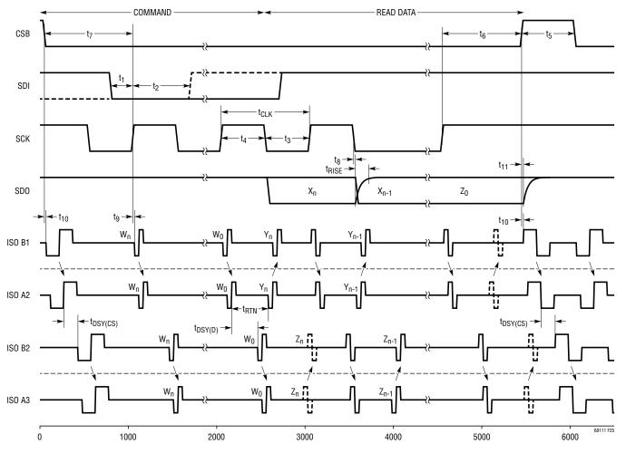
Figure 25. isoSPI Timing Diagram
