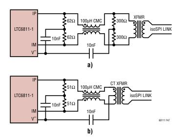
Figure 47. Daisy Chain Interface Components
