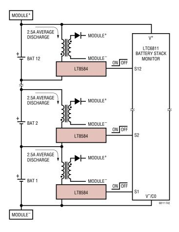
Figure 42. 12-Cell Battery Stack Module with Active Balancing
