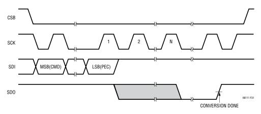
Figure 31. SDO Polling Using PLADC Command (Daisy-Chain Configuration)
