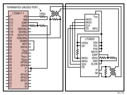
Figure 20. Single Device LTC6811-1 Using 2-Wire Port A
