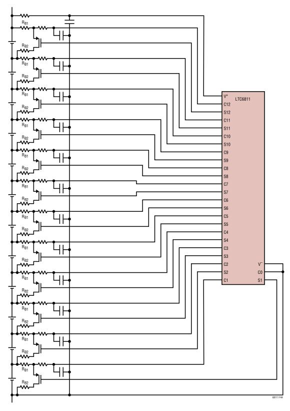
Figure 44. Balancing Self Test Circuit
