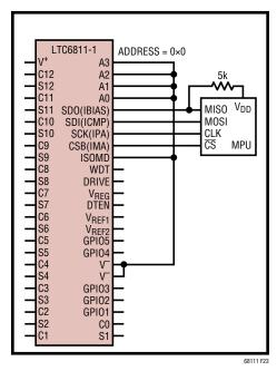
Figure 23. Single Device LTC6811-2 Using 4-Wire Port A
