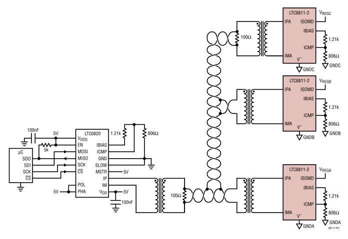
Figure 51. Connecting the LTC6811-2 in a Multi-Drop Configuration
