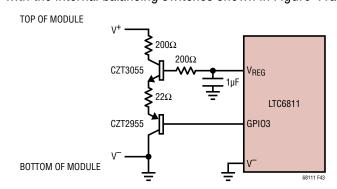
Figure 43. 200mA Module Balancer
