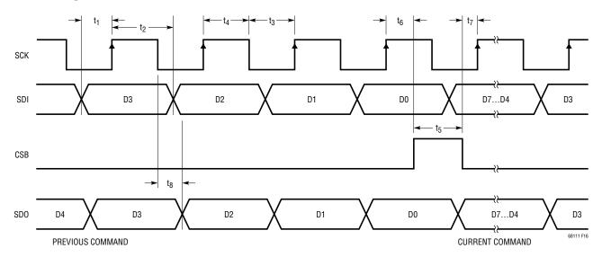
Figure 16. Timing Diagram of 4-Wire Serial Peripheral Interface
