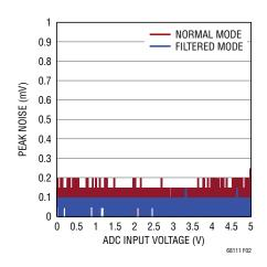
Figure 2. Measurement Noise vs Input Voltage
