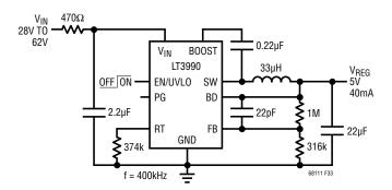
Figure 33. V<sub>REG</sub> Powered From Cell Stack with High Efficiency Regulator
