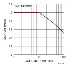
Figure 46. Data Rate vs Cable Length
