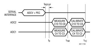
Figure 4. Timing for ADCV Command Measuring 2 Cells
