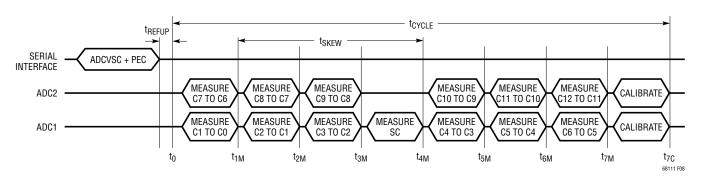
Figure 8. Timing for ADCVSC Command Measuring All 12 Cells, SC
