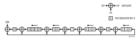
Figure 27. 15-Bit PEC Computation Circuit
