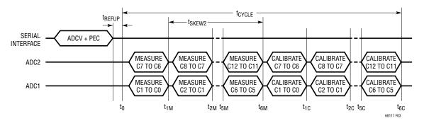
Figure 3. Timing for ADCV Command Measuring All 12 Cells
