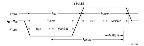
Figure 24. isoSPI Pulse Detail
