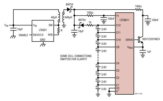
Figure 36. Flyback Converter to Power V+ and V<sub>REG</sub>
