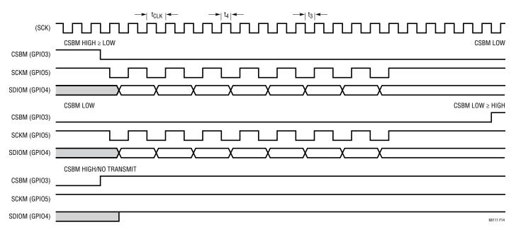
Figure 14. STCOMM Timing Diagram for a SPI Master
