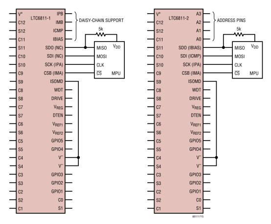
Figure 15. 4-Wire SPI Configuration
