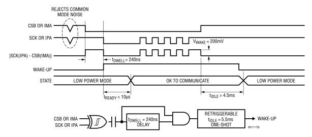
Figure 26. Wake-Up Detection and IDLE Timer
