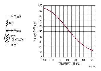
Figure 57. Typical Temperature Probe Circuit and Relative Output
