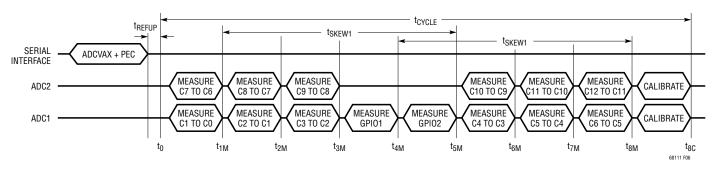
Figure 6. Timing of ADCVAX Command
