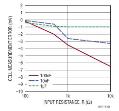
(b) Cell Measurement Error vs Input RC Values (Extra Conversion and Delay Before Measurement)
