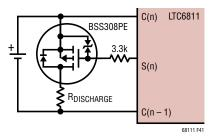
b) External Discharge Circuit
