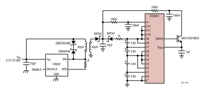
Figure 54. Powering the LTC6811 When Monitoring 4 Cells
