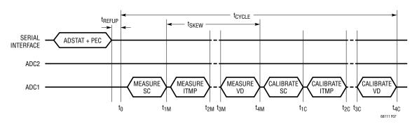
Figure 7. Timing for ADSTAT Command Measuring SC, ITMP, VA, VD
