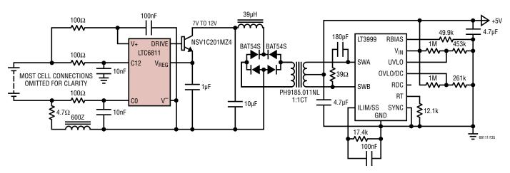
Figure 35. Push-Pull DC/DC Converter Circuit to Power V<sub>REG</sub>
