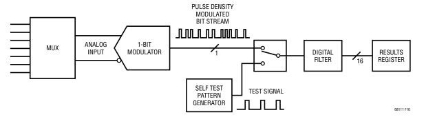
Figure 10. Operation of LTC6811 ADC Self Test
