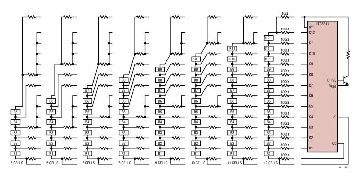
Figure 53. Cell Connection Schemes for 5 to 12 Cells
