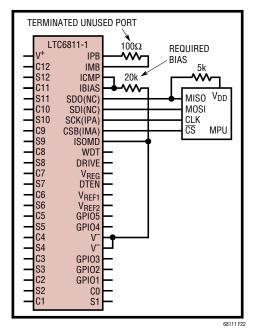
Figure 22. Single Device LTC6811-1 Using 4-Wire Port A
