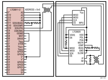
Figure 21. Single Device LTC6811-2 Using 2-Wire Port A
