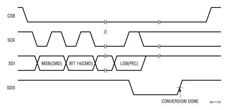
Figure 29. SDO Polling Using PLADC Command (Parallel Configuration)
