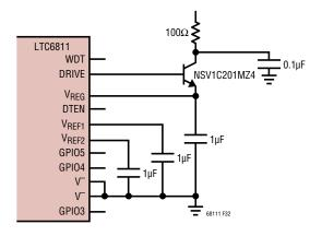
Figure 32. Simple V<sub>REG</sub> Power Source Using NPN Pass Transistor
