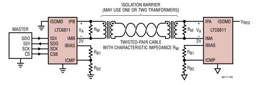
Figure 45. isoSPI Circuit
