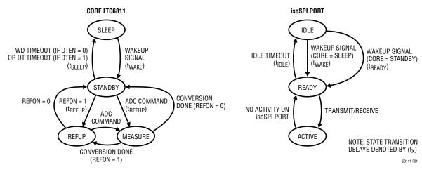
Figure 1. LTC6811 Operation State Diagram
