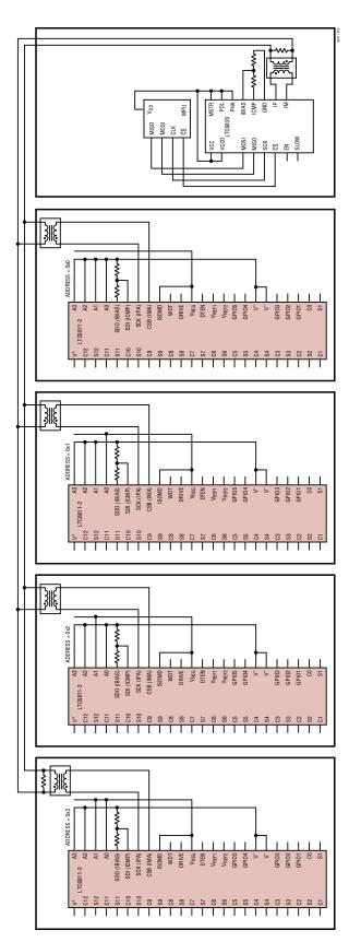
Figure 19. Multi-Drop Configuration Using LTC6811-2
