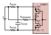
a) Internal Discharge Circuit
