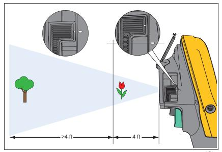
Figure 1. IR-OptiFlex Focus
