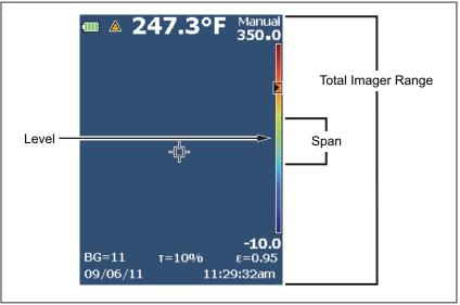
Figure 3. Level and Span Settings
