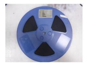
2. Seal the labeled reel in a vacuum and dry package.
