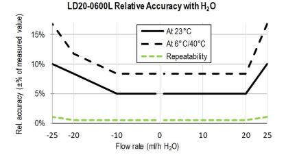
Figure 1: Liquid flow sensor accuracy and repeatability across the flow range of the LD20-0600L. Relative error in  $\pm$ % of measured value for H<sub>2</sub>O.
