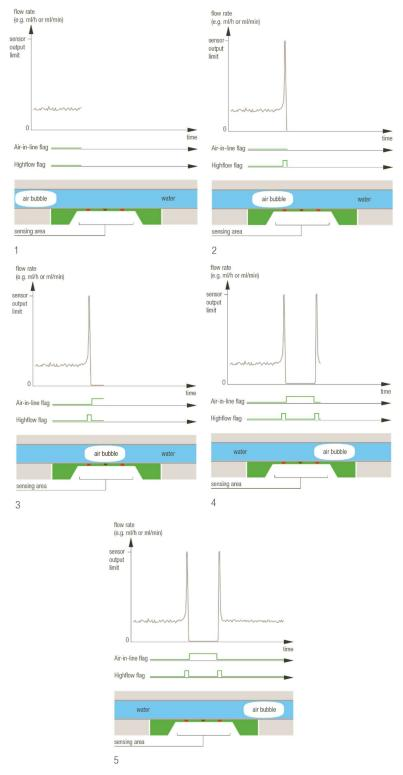
Figure 3: Detection of air-in-line events with the LD20-0600L. The graphs illustrate the air-in-line and high-flow flags while a bubble is passing though the sensor from left to right.
