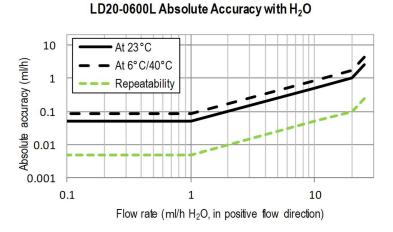
Figure 2: Liquid flow sensor accuracy and repeatability across the positive flow range of the LD20-0600L. Absolute error in ml/h for H2O.
