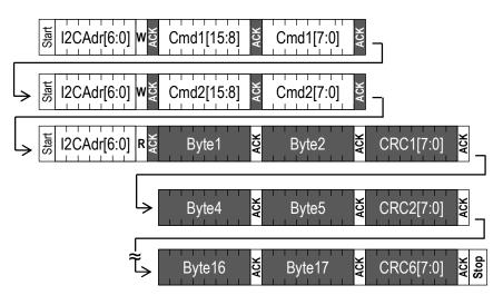
Dark areas with white text indicate that the sensor controls the SDA (Data) line.
