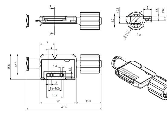
Figure 4: Preliminary dimensions of LD20-0600L (all dimensions in mm)
