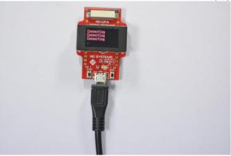
Figure 1. Connection of an IoD-09TH Display module to 4D-UPA with a microUSB Cable.
