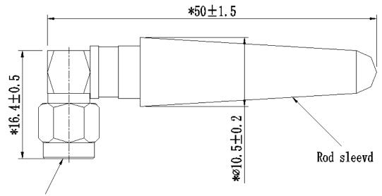
SMA/Au-PLATED (Male pin with internal thread) Salt spray requirements: ≥48h
