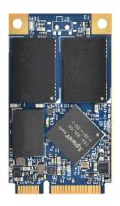
SV240-300 utilizes 3D NAND for higher capacity up to 960GB and provides more power efficiency than 2D NAND. Regarding reliability, SV240-300 is implemented with LDPC (Low Density Parity Check) ECC engine to extend SSD endurance and increase data reliability while reading raw data inside a flash chip. In addition, the drive comes with various implementations including powerful hardware ECC engine, power saving modes, wear leveling, flash block management, S.M.A.R.T., TRIM, and DataDefender™.
