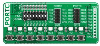
Figure 10-1: I/O group contains PORT headers, tri-state pull up/down DIP switch, buttons and LEDs all in one place
