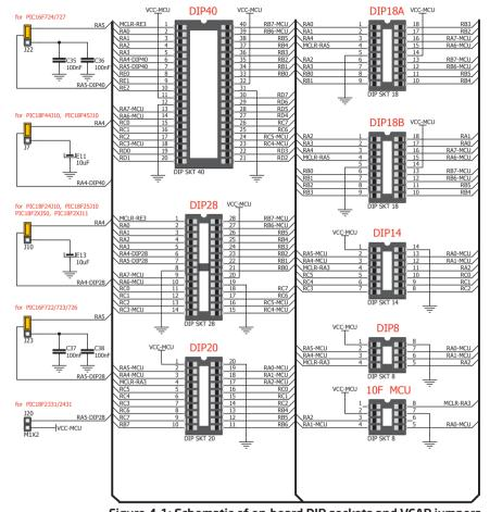
Figure 4-1: Schematic of on-board DIP sockets and VCAP jumpers
