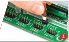
Figure 13-1: Put Touch panel flat cable in the connector
