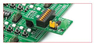
Figure 10-4: IDC10 male headers enable easy connection with MikroElektronika accessory boards
