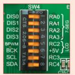
Figure 18-1: Activate SW4.7 and SW4.8 switches to connect microcontroller I<sup>2</sup>C lines to Serial EEPROM.
