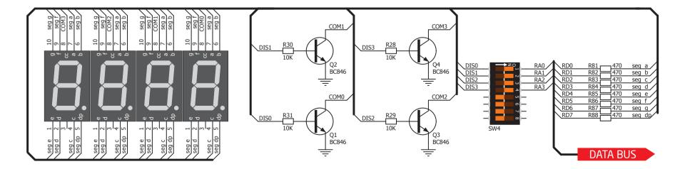
Figure 14-2: 4-digit 7-segment display schematic
