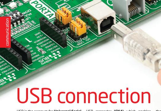
USB is the acronym for **Universal Serial Bus**. This is a very popular industry standard that defines cables, connectors and protocols used for communication and power supply between computers and other devices. EasyPIC<sup>™</sup> v7 contains
