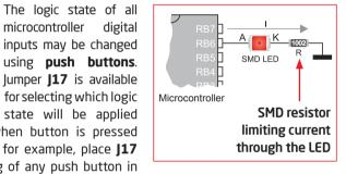
**LED (Light-Emitting Diode)** is a highly efficient electronic light source. When connecting LEDs, it is necessary to place a current limiting resistor in series so that LEDs are provided with the
