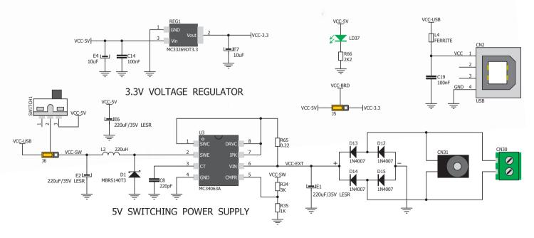
Figure 3-2: Dual power supply unit schematic
