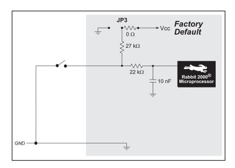
Figure 7. OP7200 Digital Inputs [Pulled Up—Factory Default]
