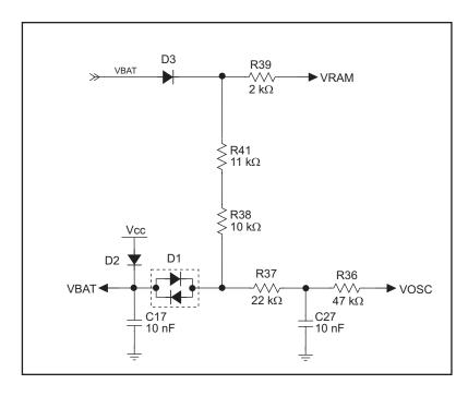
Figure B-3. OP7200 Backup Battery Circuit
