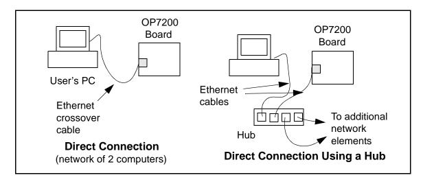
Figure 22. Ethernet Connections
