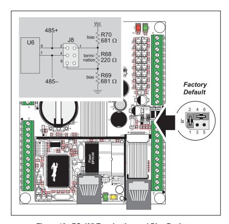
Figure 16. RS-485 Termination and Bias Resistors
