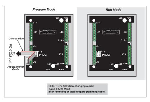
Figure 21. OP7200 Program Mode and Run Mode Set-Up
