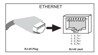
Figure 17. RJ-45 Ethernet Port Pinout
