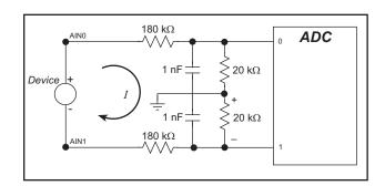
Figure 12. Current Flow from Ungrounded or Floating Source
