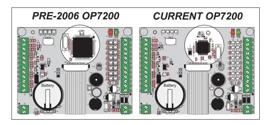
Figure 19. How to Identify Pre-2006 OP7200 Boards
