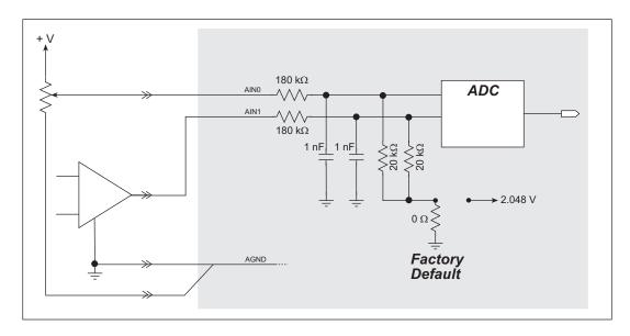
Figure 11. A/D Converter Inputs
