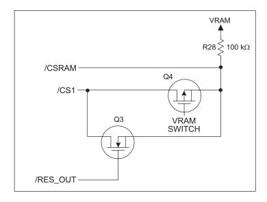
Figure B-5. Chip Select Circuit
