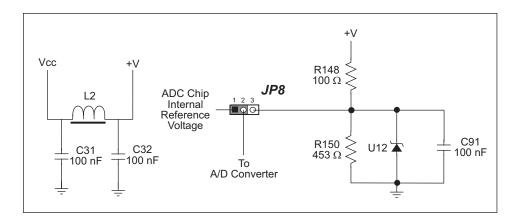
Figure 14. Analog Supply and Voltage Reference Circuits
