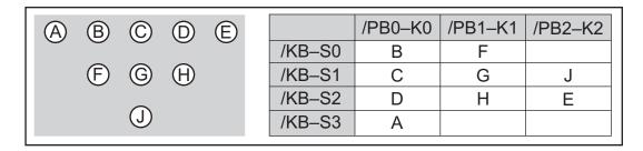
Figure 20. OP7200 Keypad Encoding
