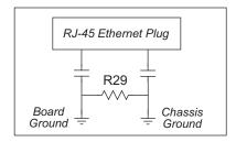
Figure 18. Isolation Resistor R29
