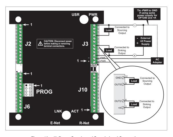
Figure 10. +K, Power Supply, and Sample Load Connections
