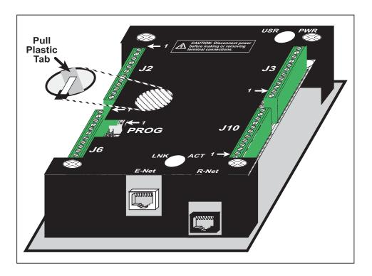
Figure 4. Remove Battery Tab
