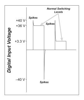
Figure 8. OP7200 Digital Input Protected Range
