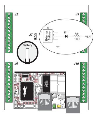
Figure B-2. OP7200 External Battery Connections
