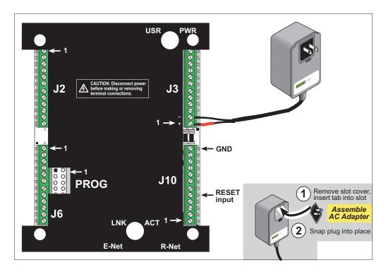
Figure 2. Power Supply Connections
