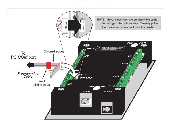
Figure 3. Programming Cable Connections
