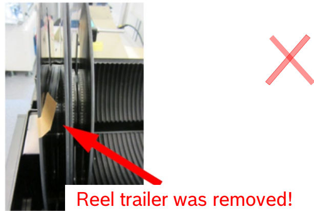
Figure 18: Reel trailers must not be removed
