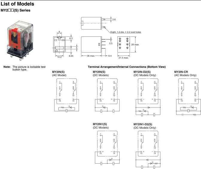
Note: For the DC models, check the coil polarity when wiring and wire all connections correctly.
