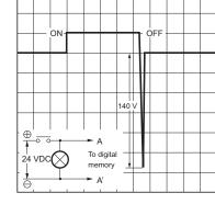
The release time will increase, but the 20-ms specification for standard models is satisfied. Diode properties:The diode has a reversed dielectric strength of 1,000 V. Forward current: 1 A
