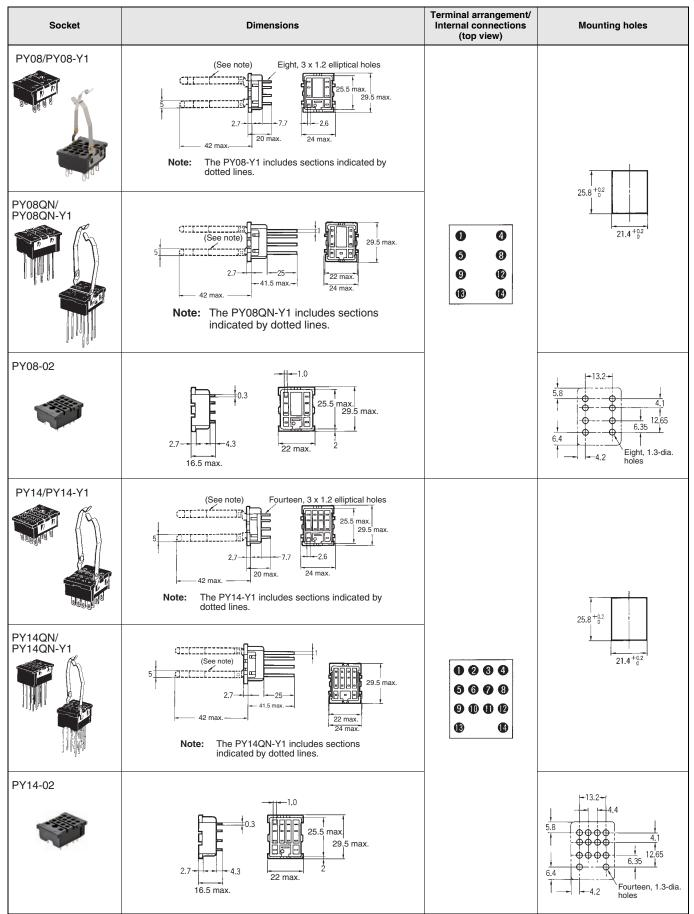
Note: Use a panel with plate thickness of 1 to 2 mm for mounting the Sockets.
