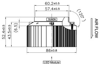
Assembly direction of customer's LED Module
