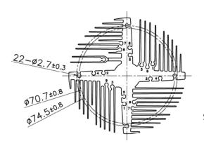
For LED Module Assembly Screw torque max 12kgf.cm
