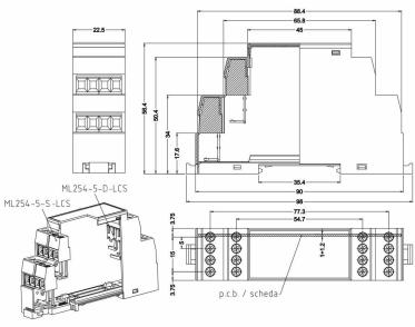
CEM22 electronic housing is realized for connections up to 16 poles.
