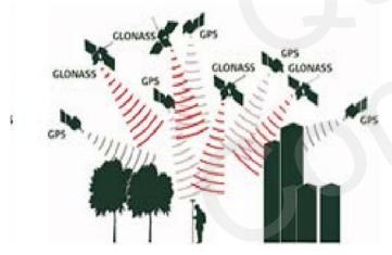
In the open sky, natural obstacles, such as trees, high buildings and etc. affects GPS modules to receive signals from satellites. The GNSS system can observes more satellites than single GPS system, which highly avoid the limitation of signal reception in the open sky.
