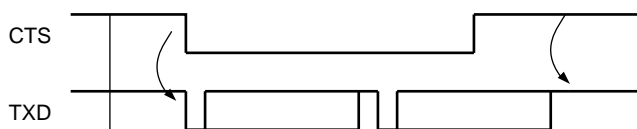
Figure 37-29. Transmitter Behavior when Operating with Hardware Handshaking
