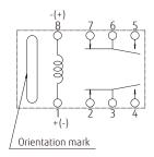
PC board mounting pad layout (TOP VIEW)
