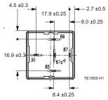
For the make contact (2x87), pin 87a = 87; for the double make contact, pin 87a = 87b.
