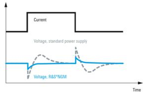
Under challenging load conditions, most power supplies respond with slow recovery times and overshoots. Specially developed circuits in the R&S°NGM200 power supplies achieve a load recovery time of <  $30 \ \mu s$  with minimal overshoot, making them perfect for supplying sensitive components.
