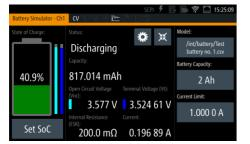
The charging behavior of a battery can also be simulated, for example when designing battery chargers. In this application, the R&S®NGM200 is used in sink mode.
