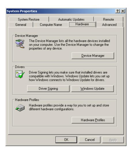
2. Expand **Universal Serial Bus Controllers**, find **Enhanced Host Controller**, and right click and select Disable it. By doing so, the USB 2.0 driver is disabled and will support USB 1.1.
