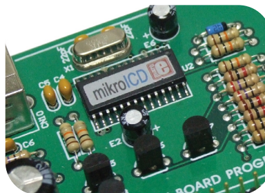
Figure 13. On-Board USB programmer
