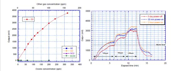
Fig. 3 Monitor sensitivity characteristics (Output range: 0 to 5V)
