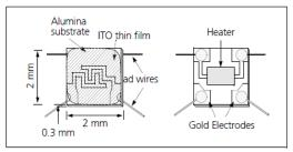
Fig. 1 Sensing Elements
