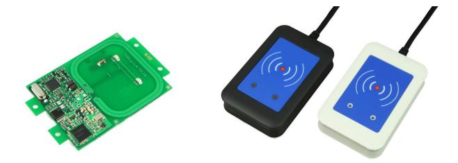
The TWN3 Legic NFC transponder reader is designed for easy integration into various applications.
