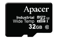
The MicroSD 5.1 card comes with 8-pin interface, designed to operate at maximum operating frequency of 50MHz or 100MHz. It can alternate communication protocol between the SD mode and SPI mode and is backward compatible with SD 2.0 devices. It performs data error detection and correction with very low power consumption.
