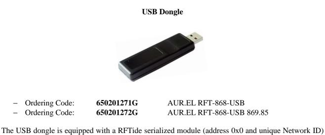
The USB dongle is equipped with a RFTide serialized module (address 0x0 and unique Network ID) and allows the module itself to be used with PC with no need for further components. In this case a virtual COM port is added to PC peripherals and, if needed, drivers are available at <u>http://www.ftdichip.com/Drivers/VCP.htm</u>.
