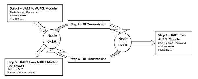
A communication is started through the issue of a generic command through the UART from the external microcontroller to Aurel module. The packet is delivered through the network to the destination node and it is redirected to UART. Successively a answer packet (Command: **ANSWER**, with a specific answer payload) returns to the first node and it is also redirected to UART.
