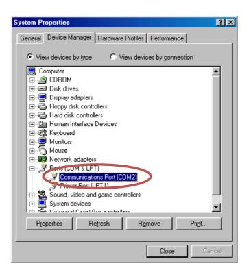
Open RFTide software, select correct COM port and press **Set** button. Next time the software is executed it tries to use the last used COM port if available. In the status bar in the lower part of the windows the current status is displayed (Current COM port or no active connection)
