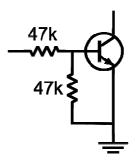
In order to reduce power consumption when the module is switched off take care of the input/output state at power-down, thus avoiding undesired current flow on the bias resistors. Similarly to +3V if a button is to be used add a pull-up (or pull-down) resistor properly.
