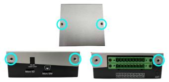
**Step 2.** Open the antenna hole by removing the cover on the hole located on the left side.
