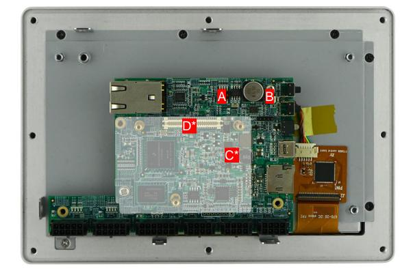
Rear view (opened device) without the Power Expansion module:
