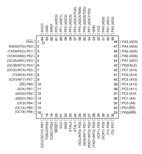
Note: The bottom pad under the QFN/MLF package should be soldered to ground.
