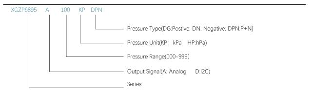
Note: 1. Voltage 5Vdc as default value, add 33(or 30) behind model signify 3.3V(or 3.0V) power supply, e.g.: XGZP6895A050KPDG33.
