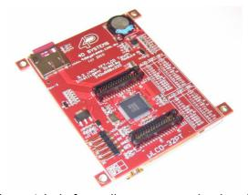
The serial platform allows users to develop their application using their favourite micro-controller and software development tools. In short, the uLCD-32PT(SGC) display module offers some of the most flexible embedded graphics solutions available.
