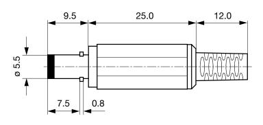
Cable diameter max. 4.0 mm
