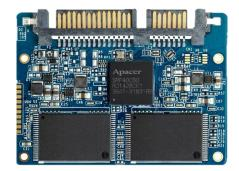
In regard of reliability, the drive comes with various implementations including powerful hardware ECC engine, power saving modes, wear leveling, flash block management, S.M.A.R.T., TRIM, and power failure management.
