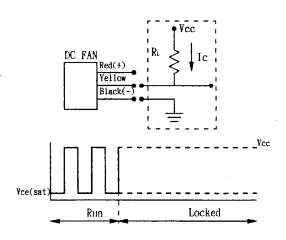
Vcc = FAN Vcc Ic = 5mA MAX Ic=VCC/RL
