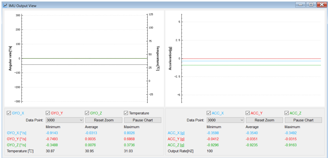
Figure 6: IMU Output – Stable Angular Rate, Acceleration, and Temperature
