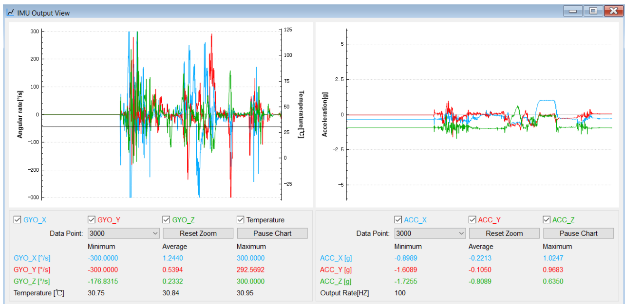
Figure 7: IMU Output – Varying Angular Rate, Acceleration, and Temperature
