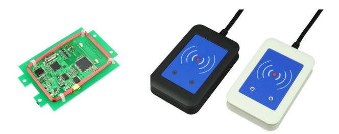
The TWN3 HID PROX transponder reader is designed for easy integration into various applications.
